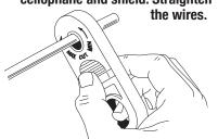
**Determine whether** you will be using the T568A or T568B configuration (above) and organize wires accordingly.
